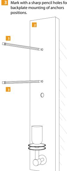
Screw in provided heavy duty Self tapping EZ anchors.
