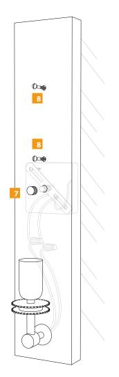
9 Screw in provided screws into anchors, DO NOT OVER TIGHTEN Just flush and snug tight is necessary.
